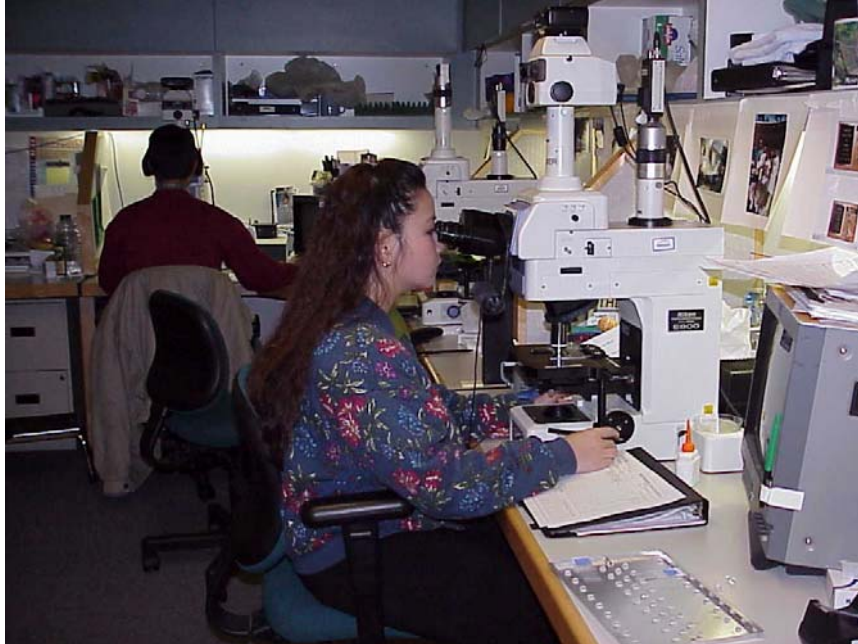
Figure 1.2 Another technologist at work in the Microscopy room. She is using the microscope to count instead of the monitor and documenting her results. Microscopy often fosters forward head posture. The Harter chair armrest does not provide adequate arm support for upper extremities despite offering height and depth adjustment. The stage control has been modified and dropped closer to the surface to reduce forward reach. The binder acts as a document support while the forearm rests on the hard surface edge.
